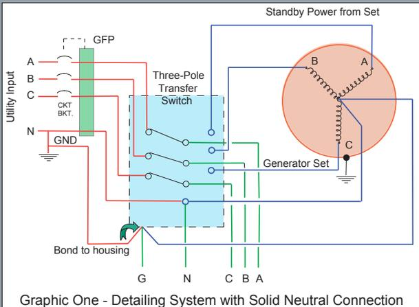
**Summary:** The general rule is when you have a grounded neutral at both the generator and the utility, you must use a transfer switch with enough poles to switch the neutral. If you ground the neutral in both places, you create undesirable multiple paths for ground current to flow.
